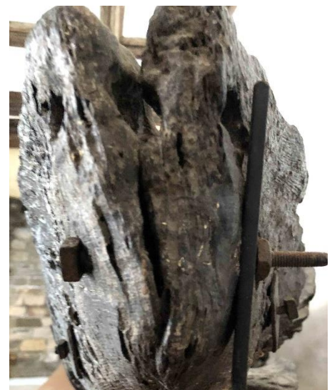
Figure 6 Splitting along the rays at the more complete end. The centre of the tree is at the bottom.
