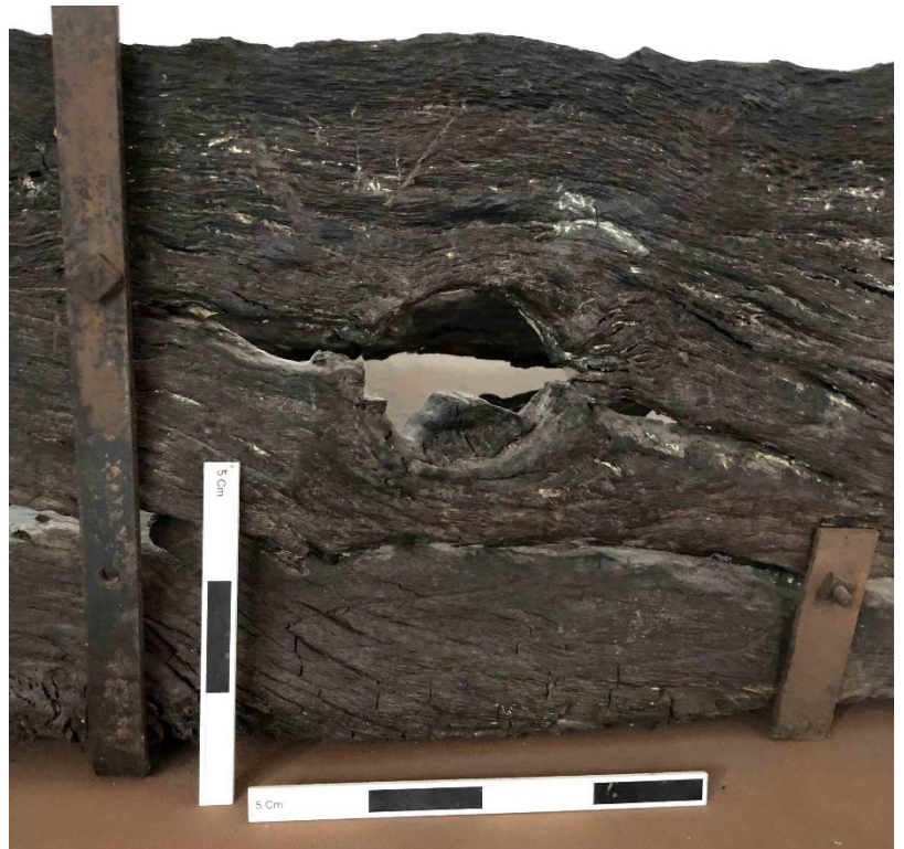
Figure 5 Knothole with remains of the side branch wood still in situ. The spiralling of the grain is visible.
